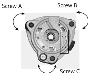
Turn the instrument approximately 90°. Adjust screw C, till the bubble in the center of the level.
