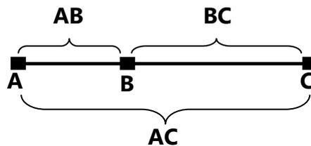
1. Select a point B on the approximately horizontal line AC with about 100 meters long. Measure the distances of lines AB, AC and BC.
