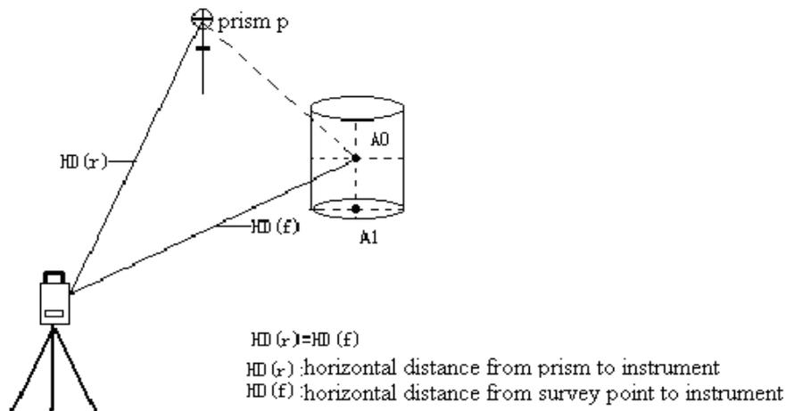
Under angle offset measurement mode, there are two methods to set vertical angle:
