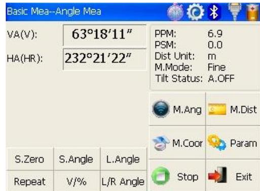
Click [V/%] key. The angles are shown in percentage values. It is possible to measure angles smaller or equal to  $\pm 45^\circ$ , otherwise "Overlay" appears on the display. 0 is set when the objective is turned in the horizontal direction:  $\pm 45^\circ = \pm 100\%$ , Horizontal=0°.
