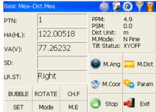
When you preset the measuring times, the instrument will carry out distance measurement and display the average distance according to the setting times. If you preset single observation (Fine mode), the average distance won't be displayed, but the distance comes out from a single measure.
