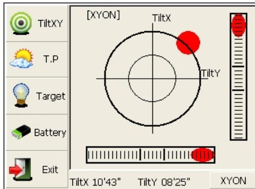
Firstly, press the [★] key to turn on the electronic bubble as shown in left figure.
