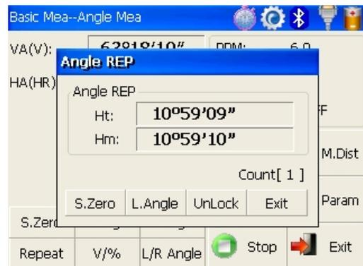
Collimate the first target A again using horizontal clamp and tangent part.
