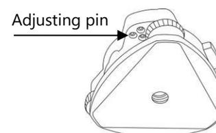
**NOTE:** Be careful when adjusting the three screws, and the tightening tension is identical for them.
