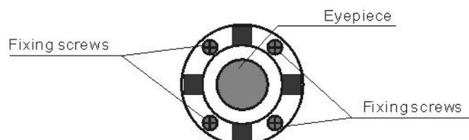
**NOTE:** After the adjustment of cross-hair, please check the collimation error and vertical index error, see 8.7. EDM optical axis and the telescope sighting axis error.
