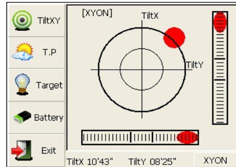
**T.P.:** observation and setting of temperature and atmospheric pressure
