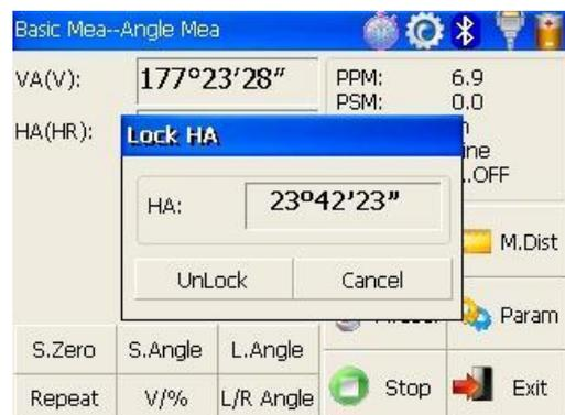
Click [UnLock] key to deactivate the function of locking horizontal angle. Then the screen will return to normal angle measurement mode, and meantime horizontal angle will be set as locked angle.
