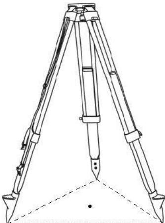
Set up the tripod first: extend the extension legs to suitable lengths and tighten the screws on the midsections. Make sure the legs are spaced at equal intervals and the head is approximately level. Set the tripod so that the head is positioned over the surveying point. Make sure the tripod shoes are firmly fixed in the ground.
