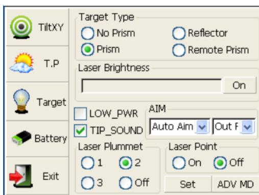
Press the [★] key and click the “target” button to enter the display shown in the figure on the left. You can turn on laser plummet and set it as three levels of brightness. Thus, that laser emits downwards can be seen.
