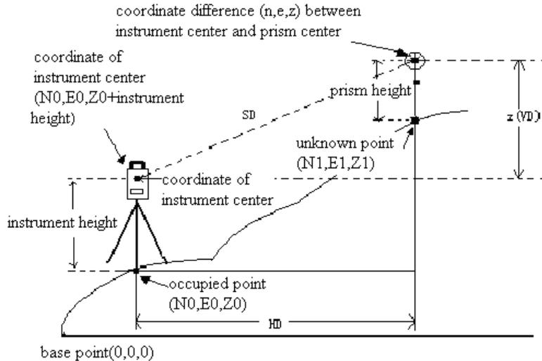
Set coordinate of occupied point (see 6.3.1. Setting coordinate of occupied point) instrument height/prism height (see 6.3.3. Setting instrument and prism heights) and backsight azimuth angle (refer to 6.3.2. Setting backsight point or 6.1.3. Setting horizontal angle to a required value). If don't input coordinate of occupied point, previous coordinate of occupied point is set as default; the same for instrument and prism heights.
