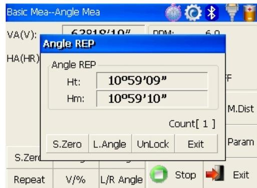
Collimate the second target B again using horizontal clamp and tangent part.
