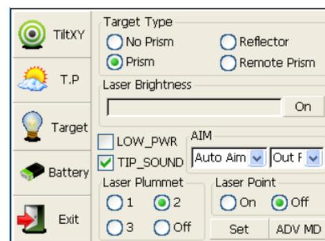
manually), **Auto Aim** (to aim it automatically) or **Lock** (to remain on the same position). In the righter box, choose if you are working indoor or outdoor.
