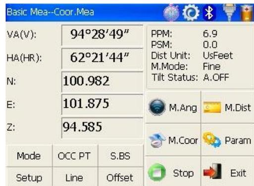
After instrument is established in P1, enter into traverse surveying of coordinate measurement through the [Setup] button and select "Call" button with stylus.
