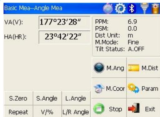
Click [L.Angle] key to activate the function of locking horizontal angle.
