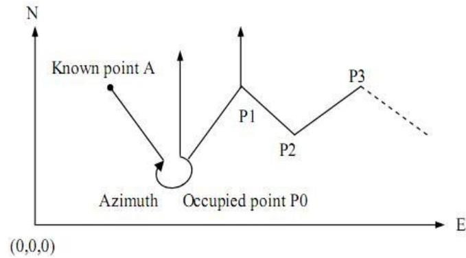
Set coordinate of occupied point P0 and azimuth angle from point P0 to known point A.
