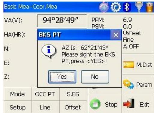
Collimate backsight point, click [Yes] key. And then the system will define backsight azimuth angle which displays in the upper left corner of coordinate measurement screen.
