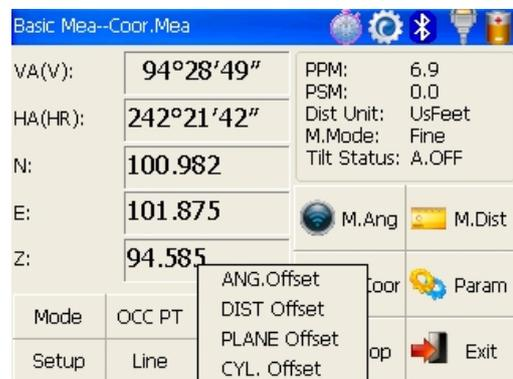
Entry the horizontal distance of front and back (**dFR**) and horizontal distance of left and right (**dRL**).
