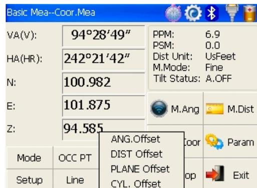
Select "Free VA" (or "Lock VA") with stylus to start angle offset measurement (user makes a choice on the basis of own demand)
