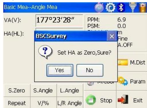
Collimate the second target, and the horizontal angle and vertical angle will display on the screen of instrument.
