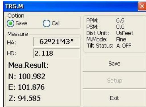
Click [Save] key. Coordinate of P1 can be ascertained and it will return to main menu. At last, power off and transfer instrument to P1 (transfer prism from P1 to P0 meantime).
