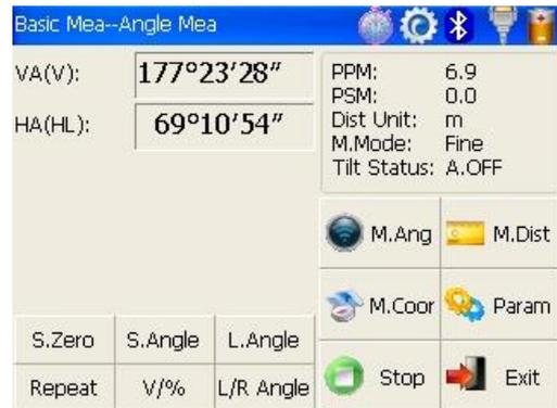
Switch horizontal angle between left and right by clicking [L/R Angle] key.
