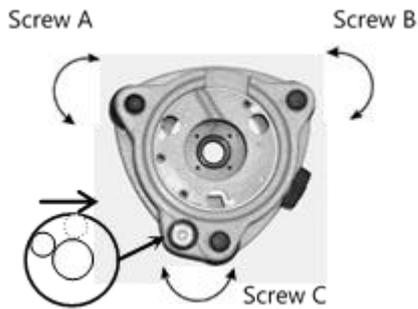
Move the foot screws A and B in opposite direction till the circular bubble is perpendicular to a line shaped with screw A and B. The direction of rotation in left thumb indicates the movement of the circular bubble.
