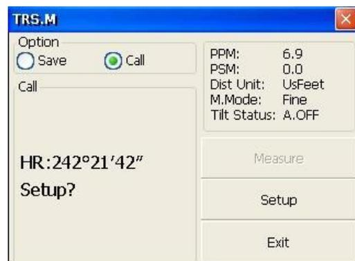
Collimate last occupied point P0. Click [Setup] key.
