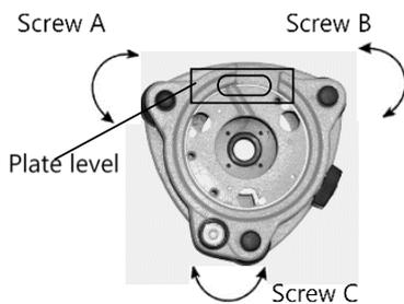
Loosen the horizontal motion clamp and turn the instrument till the plate level is parallel to a line shaped with screws A and B. Adjust the screws A and B to make the bubble in the center of the level.
