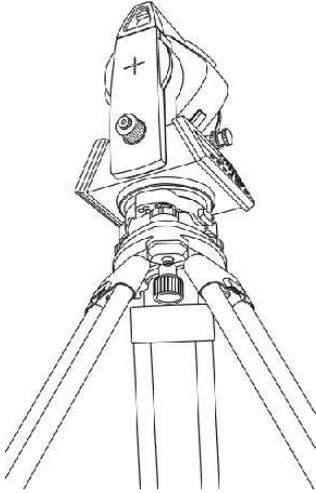
Mount the instrument on the tripod head. Supporting it with one hand, tighten the centering screw on the bottom of the unit to make sure it is secured to the tripod.
