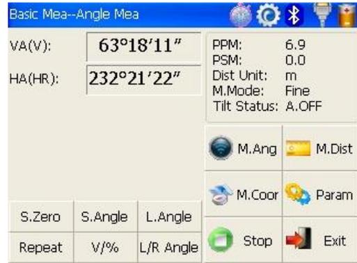
Collimate the first target A and click [S.Zero] key, and set horizontal angle as zero.
