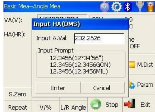
Click [Enter] key, and angle measurement after orientation will go on.
